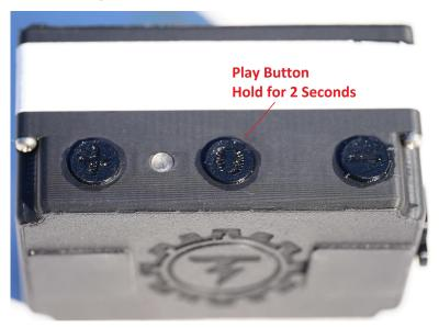
To put the Speaker in pairing mode, hold the **Play button** for about 2 seconds. You will hear a long beep, followed by the indicator light flashing white and red.
