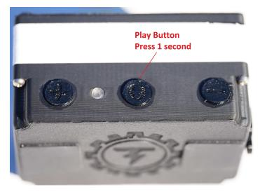
To power on hold the **Play button** for about 1 second. You will hear the speaker boot up and the indicator light Flicker three times.
