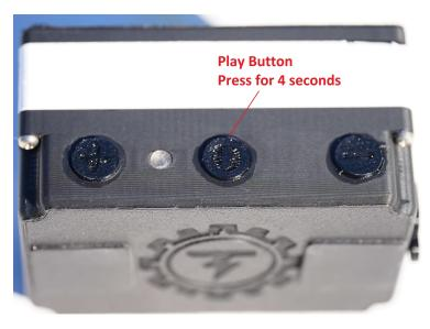
To Power off, hold **Play button** for about 4 seconds. You will hear the one beep, then the power off beep. You will need to hold the power off button until you hear the second beep.
