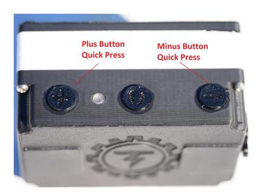
To increase the volume of the Speaker, quick press the **Plus button**. To decrease the volume of the speaker, quick press the **Minus button**.
